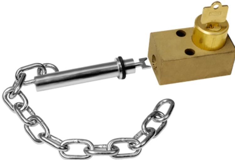
The Type DM access door interlock is designed for hinged doors, manhole covers, sliding doors or any sort of hatch or lid. It is well suited for loose fitting doors or hatches that will not accommodate a precise fitting door lock.
